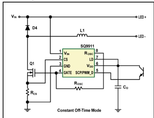
Figure 4. Typical Application Circuit without PFC in Fixed Frequency Mode
