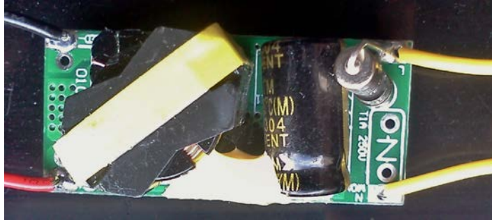
Figure 5. Top View of this Power Module
